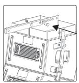
4. Insert the second clevis pin into the inner through-hole.
