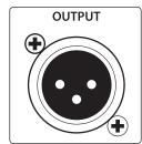
**Direct Out**. This is the Direct Out for the line input. Use this to connect to other CDL-series loudspeakers. **See Section 3.4 for a connection example.**
