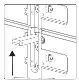
5. Insert the pin into the upper hole of the rigging clasp until it locks, and rotate it up to lock the handle in place.
