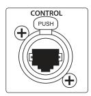
**Dante / Control**. This locking Ethernet connection can be used for control via the Worx Control application as well as Dante audio networking. A standard RJ45 connector may be used, but we recommend the protection provided by using the mating male locking Ethernet connector. For more information on creating a wired LAN network and using Dante, see the Worx Control Reference Manual.
