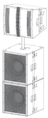
**WARNING:** Maximum pole height from the top of the upper CDL18s to the bottom of the CDL12 cannot exceed 17". PreSonus recommends the K&M 21334.050.55 Distance Rod.
