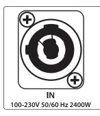
AC Line Connection. CDL-series loudspeakers have a universal power supply that accepts AC power input between 100 and 250 VAC at 50/60 Hz. Each loudspeaker is supplied with an AC powerCON® power cord appropriate for the country of sale.
