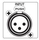
**Line Input**. This is a balanced XLR connection for line-level input. Use the Line input to connect the loudspeaker to a StudioLive digital mixer or another mixing console, either directly or through the Line out connector on a CDL-series loudspeaker.
