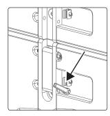
2. Press the release button to unlock the pin.
