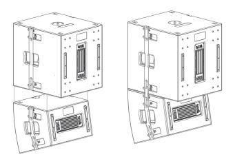
Note: CDL12 loudspeakers must be mounted to the bottommost CDL18s in a suspended vertical array. A CDL12 can be mounted atop a CDL18s for groundstacked applications only. See Section 2.8 for more information.
