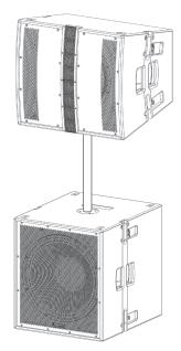
**WARNING:** Maximum pole height from the top of the CDL18s to the bottom of the CDL12 cannot exceed 40". PreSonus recommends the K&M 21339.000.55 Crank Stand.
