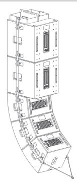
**WARNING:** The CDL Rigging Sling is required on all installations that include 4 or more CDL-series loudspeakers in a vertical array. Additionally, in installations using the CDL Rigging Extension Bar deployed with an upward or downward tilt of 12° or greater, the CDL Rigging Sling must be utilized.
