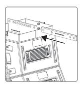
1. Align the CDL Rigging Extension Bar with the center support of the CDL Rigging Grid.
