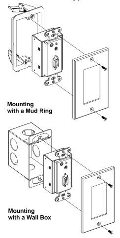
3. After making the necessary unit-to-unit Cat 5e cable connections, as well as the terminal block connection (optional), attach the Decora Face Plate to secure and cover the VE156 / VE606 / VE806.
