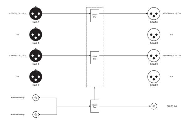
ADA4, Synchronizer Mode Block Diagram (Jumper 2 Removed), D/D
