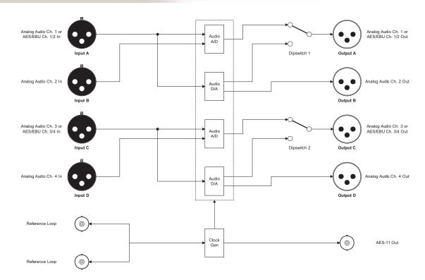
ADA4, Normal Mode Block Diagram (Jumper 2 Installed), A/D or D/A
