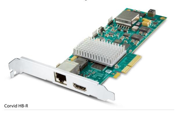
Expand your application's reach with HDBaseT and the Corvid HB-R. Using a single Cat 5e/6 cable as input, the Corvid HB-R receives up to 4K/60p video (8-bit 4:2:0) and 8-Channel embedded audio.
