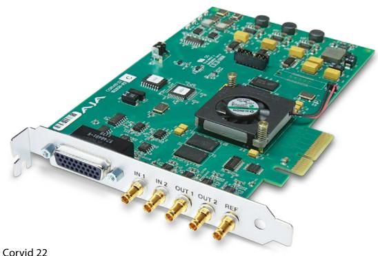
Get multiple I/O Channels without taking up a lot of space. Corvid 22 provides high performance, dual channel video and embedded 24-bit audio I/O in a single PCIe card. Two completely independent channels\* handle resolutions up to 2K and high frame rate 1080p as well. With separate LTC and RS-422 machine control per channel and support for multiple operating systems, Corvid 22 gives you all the performance and capabilities you need.
