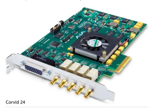
Take the next step in multi-channel video and audio I/O with Corvid 24. Corvid 24 is the intermediate solution for high density I/O, supporting up to 4 independent\* channels of capture or output, with separate LTC, embedded 24-bit audio, and metadata for each channel. Or all four connections can be used to support full 4K; the choice is yours. And with multiple operating system support, Corvid 24 will work in almost any environment.
