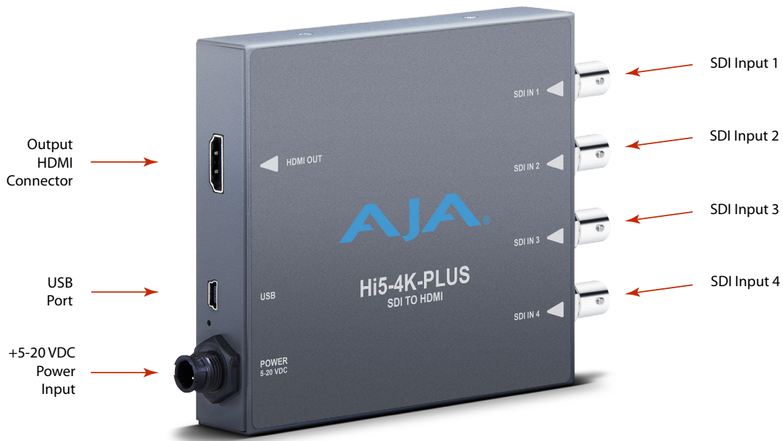
Figure 2. Hi5-4K-Plus Converter Connections
