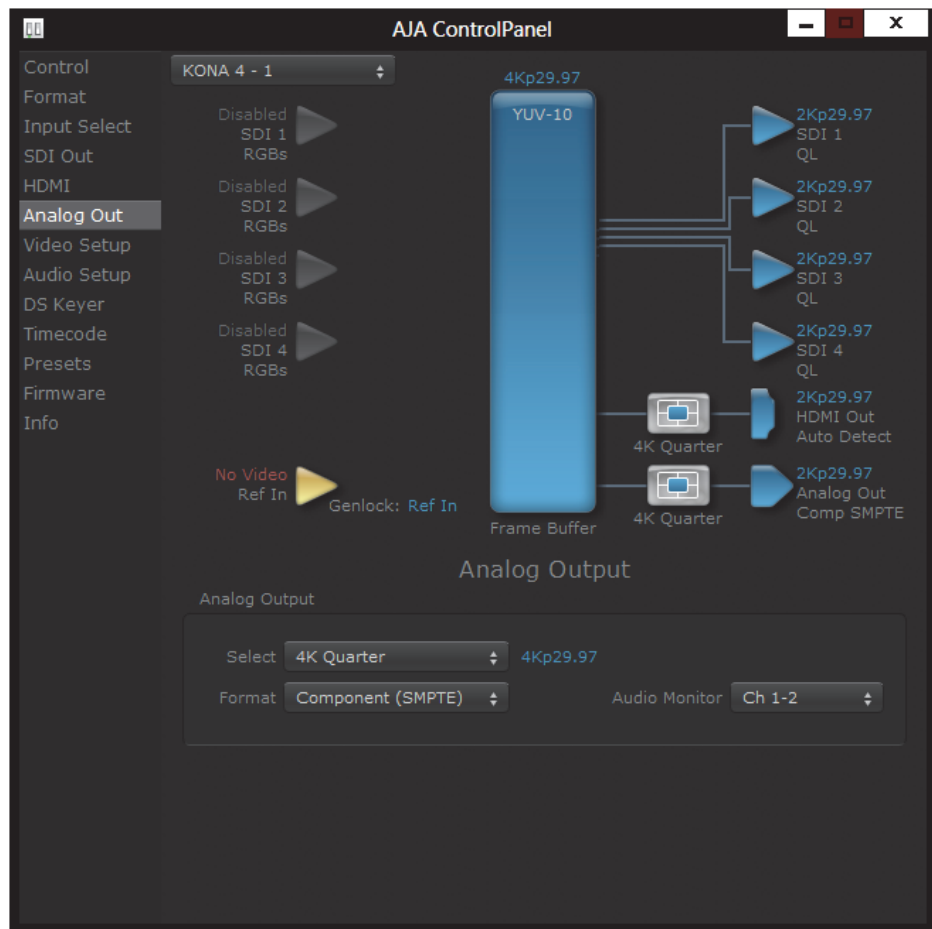
Figure 72. Analog Output Screen with 4K Primary Format
