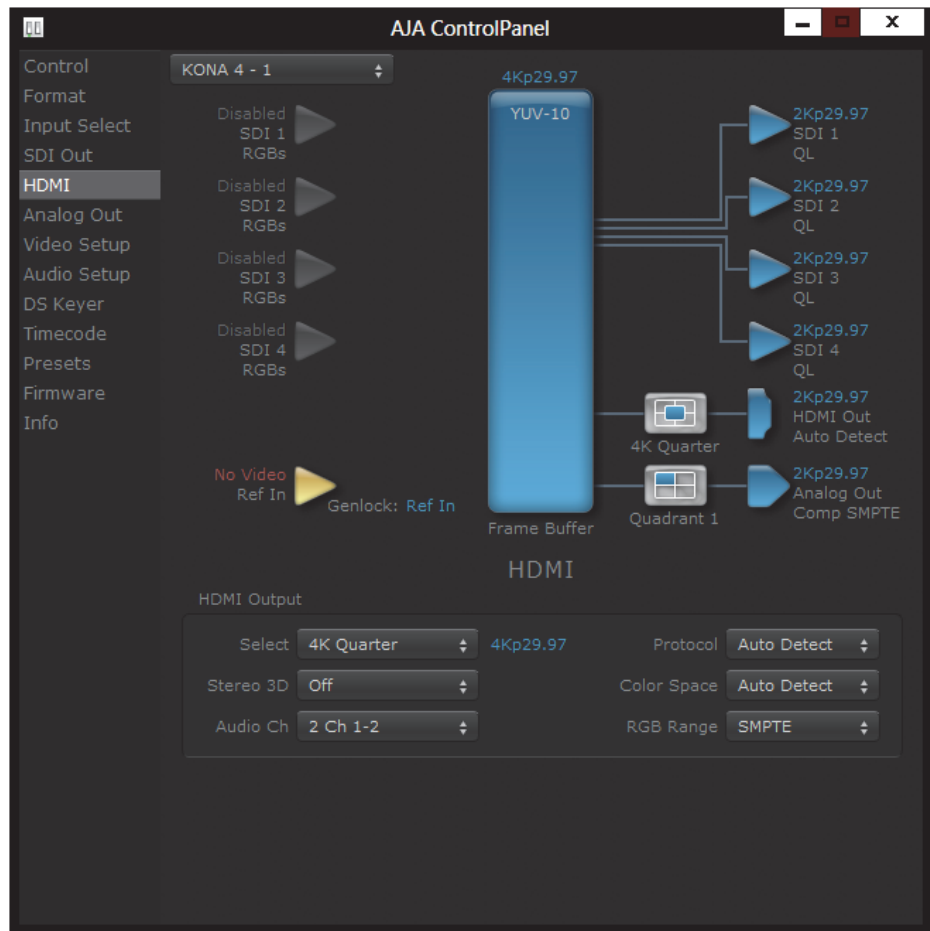
Figure 70. HDMI Output Screen with Quad HD Output Configuration
