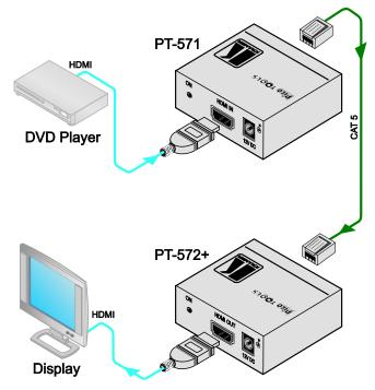
*Figure 3: Connecting the PT-571/PT-572+ HDMI Line Transmitter/Receiver*
