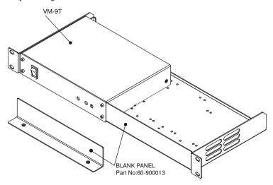
Figure 5: RK-1 Rack Adapter - Connecting a Blank Panel
