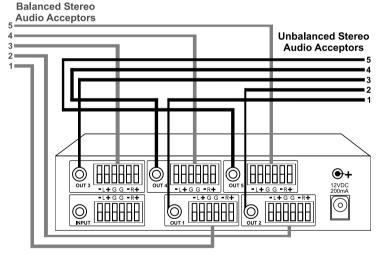
Figure 4: Connecting the VM-50AN as a 1:10 Audio Distributor
