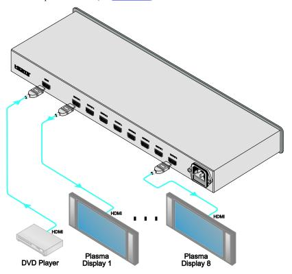
Figure 3: Connecting a VM-8H 1:8 HDMI Distributor
