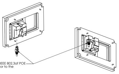
Before installation of the wall mount, connect a 48V IEEE 802.3af POE power source via a CAT5/6 cable and RJ45 connector to the POE to USB converter.
