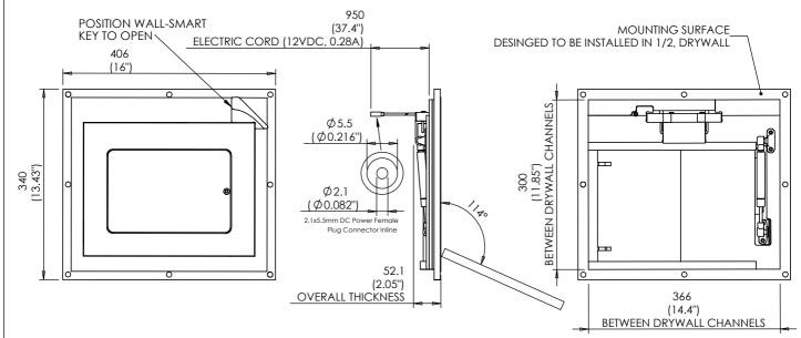
by Wall-Smart www.wall-smart.com UNLESS OTHERWISE SPECIFIED: DIMENSIONS ARE IN MILLIMETERS INFORMATION CONTAINED HEREIN IS PROPRIETARY AND MAY NOT BE USED, REPRODUCED OR COPIED WITHOUT WRITTEN CONSENT OF WALL-SMART •
