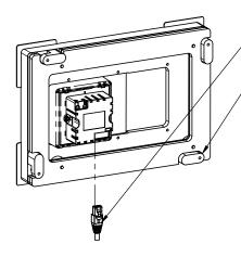
—Before installation of the wall mount, connect a 48V IEEE 802.3af POE power source via a CAT5/6 cable and RJ45 connector to the POE to USB converter.
