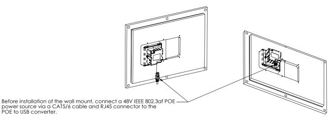
If required, it is possible to unscrew 6 screws, remove the back wall and connect POE cable after the wall mount was installed. The state of the s
