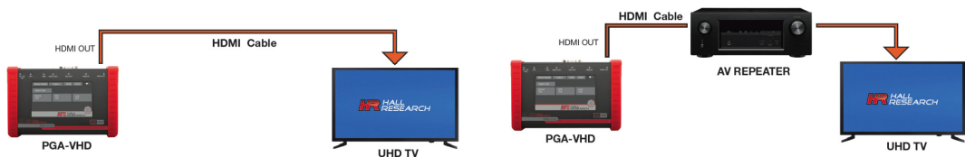
Sink Test - PGA-VHD Acting as Video Generator
