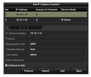
3. Select the detected IP camera and click the **Add** button to add it directly, and you can click the **Search** button to refresh the online IP camera manually.
