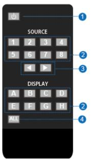
1 Press the key to open the power of the matrix
