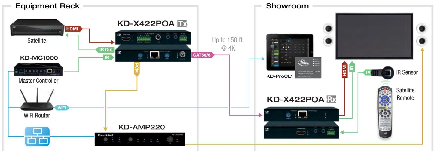
\* For all installations, we highly recommend use of KD-CAT6STP1X STP cabling, especially in hostile electrical environments. The shield of CAT6STP must be soldered on both ends to the shield of RJ45 connector used. The CAT5/5e/6 cable has to be terminated according to TIA/EIA-568-B standard. The use of STP CAT5, 5e is not recommended.
