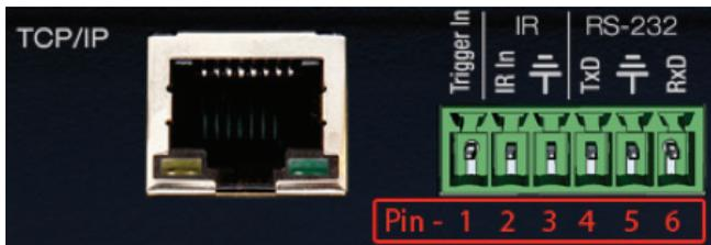
The KD-Pro2x1/KD-Pro4x1 features a 6-Pin Terminal Block for Trigger In, IR, and RS-232 Control. Signals may be received from these connections as well as the Ethernet Jack for TCP/IP Control. Serial commands may be found in the "Communications Protocol" section.
