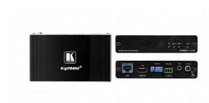
TP-583Txr is a high-performance, extended-reach HDBaseT transmitter for 4K HDR HDMI, RS-232 and IR signals over twisted pair. TP-583Txr converts all input signals into the transmitted HDBaseT signal. It enables extending video signal up to 100m (330ft) at 4K@60Hz (4:4:4) video resolution, up to 180m (590ft) at 4K@60Hz (4:2:0), and up to 200m (650ft) at HD video resolution over Kramer copper cables. It is compatible with standard HDBaseT-compliant extenders at 4K@30Hz and HD video resolutions
