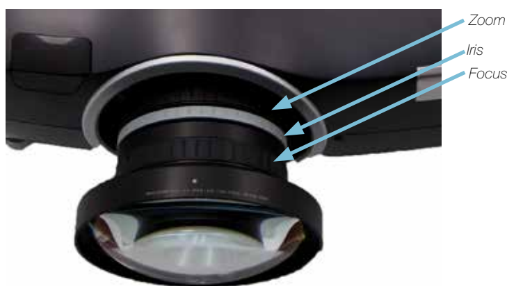
Figure 4-9. Zoom, Focus and Iris rings on the lens (may vary on some lenses)
