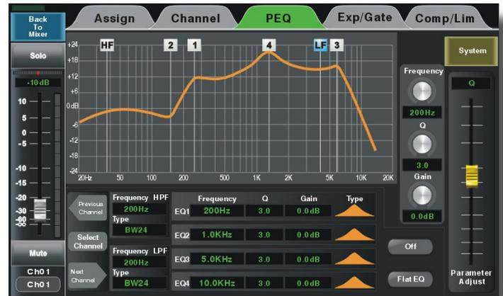
Figure 4.2: PEQ Parametric EQ Screen
