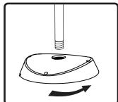
3. Thread cover plate on to conduit until secure.
