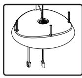
6. Slide cover plate over hanging and safety cables and run RJ45 signal wire
