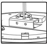
8. Extra slot and 2 holes provided for additional safety cables where needed.
