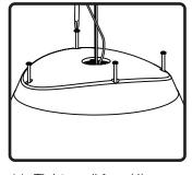
11. Tighten all four (4) screws to lock cover plate in place.
