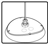
4. Tighten the top of 3/8" NPT wire gland such that the rubber grommet is tight around the cable. This may require a wrench.
