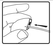
2. Thread hanging or safety cable through SpeedClamp™ mechanisms as shown.
