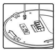
7. Plug RJ45 connector into speaker. If local power\* is required at speaker (non-POE installation), connect appropriate DC power supply to barrel connector on speaker input panel.
