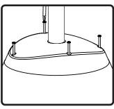
9. Tighten all four (4) screws to lock speaker in to cover
