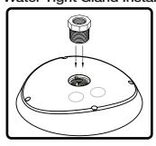
Thread the 3/4" to 3/8" NPT adapter into the the top plate of the speaker in the hole provided. Make sure to tighten securely to ensure a water tight fit.
