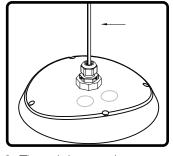
2. Thread the 3/8" NPT wire gland into the 3/4" to 3/8" rity cable and ethernet cable, NPT adapter. Make sure to prior to terminating the RJ45 connector, through the 3/8" NPT wire gland and attach to the back of the speaker as noted in previous instructions.
