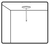
2. Securely mount conduit to structure. Conduit must have 3/4" NPT thread to accomodate RS-EZ speaker.
