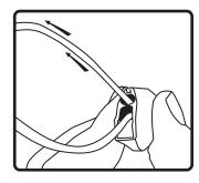
5. Adjust speaker hanging height with SpeedClamp™ mechanism. Pull to tighten & press button on SpeedClamp through center hole. as shown to loosen or adjust.
