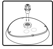
tighten securely to ensure a water tight fit.
