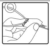
4. Thread cable end(s) through SpeedClamp™ mechanisms as shown.
