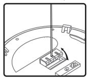
6. Align safety cable with center slot and pull up to secure.
