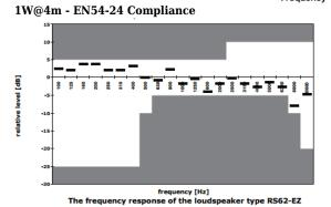
Octave band Declared coverage Measured coverage filter angle angle 500 Hz / 1W/4m 360 360 1 kHz / 1W/4m 150 150 102.5 2 kHz / 1W/4m 105 4 kHz / 1W/4m 74 70
