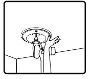
7. Insert speaker into mounting hole with paint mask in place. Tighten both screws on the baffle face to actuate the mounting wings. Firmly secure both screws. DO NOT OVERTIGHTEN.
