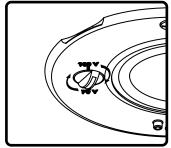
9. Adjust tap switch to proper setting. Switch is preset to 8 Ohm mode.
