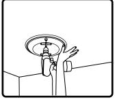
6. Insert speaker into mounting hole with paint mask in place. Tighten both screws on the baffle face to actuate the mounting wings. Firmly secure both screws. DO NOT OVERTIGHTEN.
