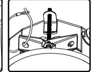
6. If required, attach seismic restraint system to hole in clamping arm, then to reinforced structure (saftey cable not included)
