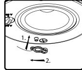
10. Attach grille safety clip by placing the large end of the clip over snap-fit post (1), then sliding clip until small end snaps into place around post (2).
