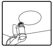
3. Use RotoZip or other tool to cut hole. Hole diameter: 5.6 in.
