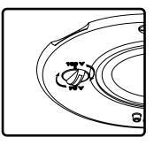
8. Adjust tap switch to proper setting. Switch is preset to 8 Ohm mode.
