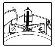
5. If required, attach seismic restraint system to hole in clamping arm, then to reinforced structure (saftey cable not included)
