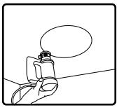
3. Use RotoZip or other tool to cut hole. Hole diameter: 5.6 in.
