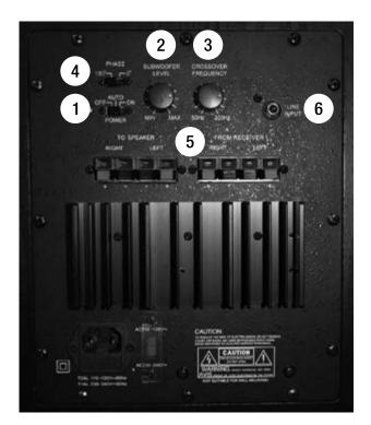
**1. Power ON/Auto/OFF:** This switch, when left in the "Auto" position, automatically activates the subwoofer when an audio signal is detected and shuts the subwoofer off after approximately ten (10) minutes of silence.
