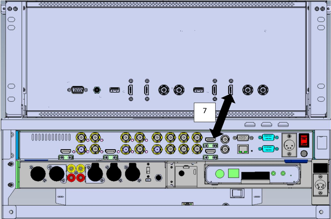
3. Please connect the Cable No. 8 (HDMI Cable) from the PGM HDMI OUT interface on the rear panel of the KMU-100 to the HDMI IN interface on the rear panel of the NVS-30.
