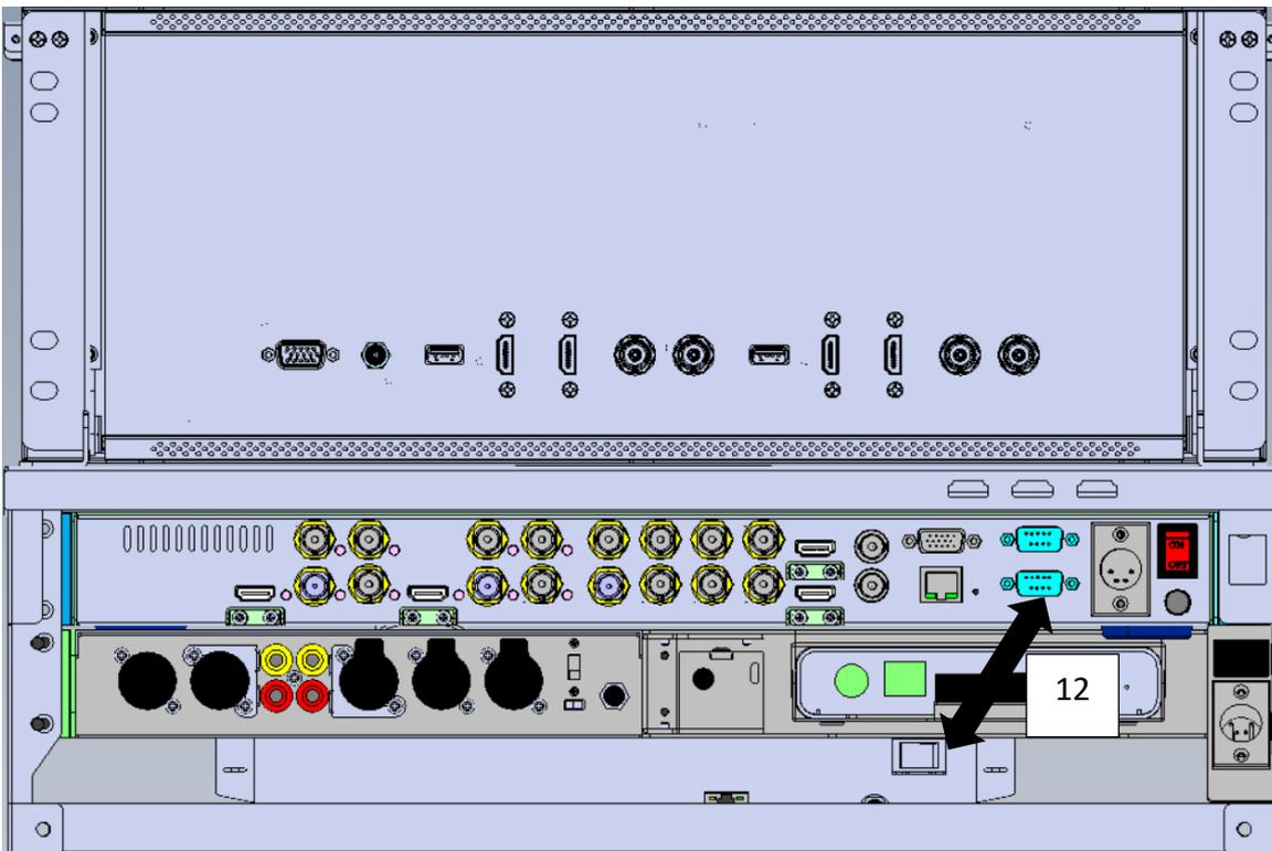
8. First locate the DC jack on the RMK-6 and on the inner side of the DC jack, you should find five DC plug cables attached. Connect Cable No. 1 / 2 / 3 / 4/5 (DC Plug Cable) to the RMC-185, TLM-102, AD-100M, NVS-30 and KMU-100 DC jacks respectively and secure by tightening the outer fastening ring.
