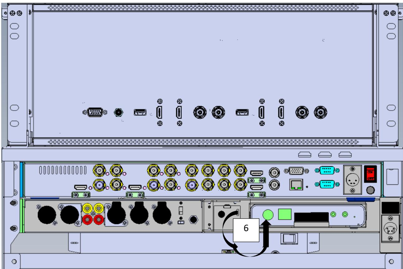
2. Please connect the Cable No.7 (HDMI Cable) from the Multiview HDMI OUT interface on the rear panel of the KMU-100 to the HDMI IN1 interface on the rear panel of the TLM-102.
