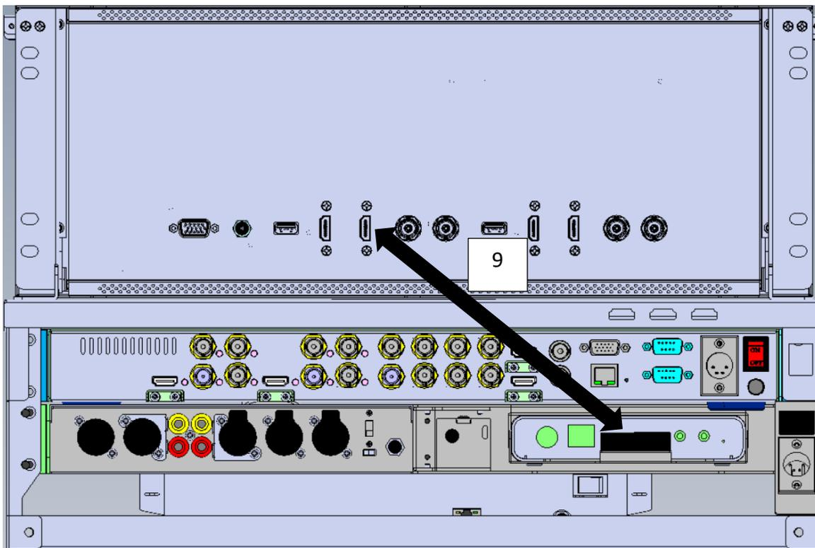
5. Please connect the Cable No. 10 (RCA Cable) from the RCA output interface on the rear panel of the AD-100M to the 3.5mm unbalanced analog audio input interface on the rear panel of the NVS-30.
