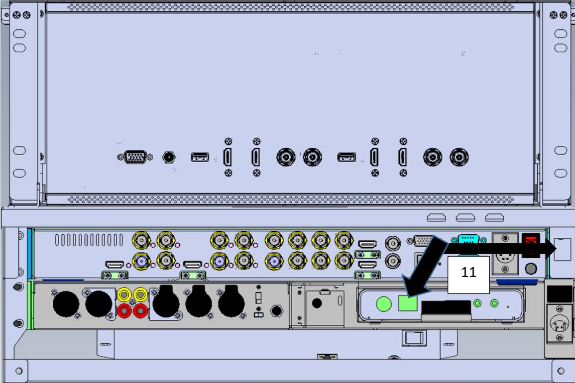
7. Please connect Cable No. 12 (RS-422 to RJ-45 adapter cable) from the RS-422 interface on the rear panel of the KMU-100 to the RJ-45 interface on the rear panel of the RMC-185.
