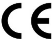
**CE Marking** is the symbol as shown on the left of this page. The letters "CE" are the abbreviation of French phrase "Conformité Européene" which literally means "European Conformity". The term initially used was "EC Mark" and it was officially replaced by "CE Marking" in the Directive 93/68/EEC in 1993. "CE Marking" is now used in all EU official documents.
