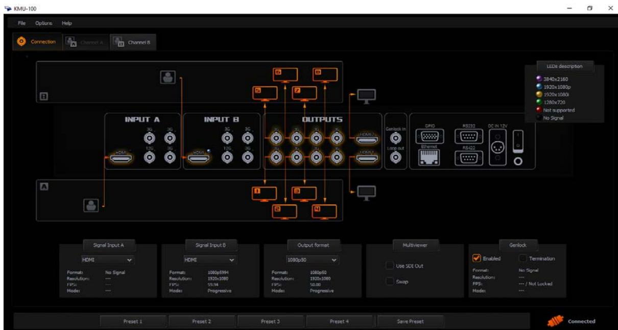
The Connection tab allows you to define input signals connected to **Channel A** and **Channel B**. It is also possible to use the signal from **Input A** to process in **Channel B**, and vice versa, i.e. processing of **Input B** in **Channel A**.
