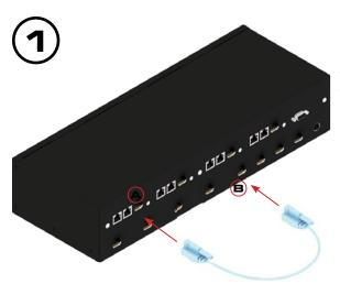
This example shows the jumper connection between HDMI output port 1 and HDMI extension input port 1 .
