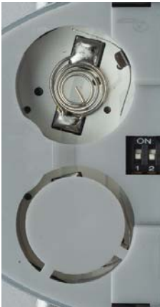
Left: Picture of the opened rear battery compartment of the RMT-16IR remote showing the exposed DIP Switch bank between the battery chambers.
