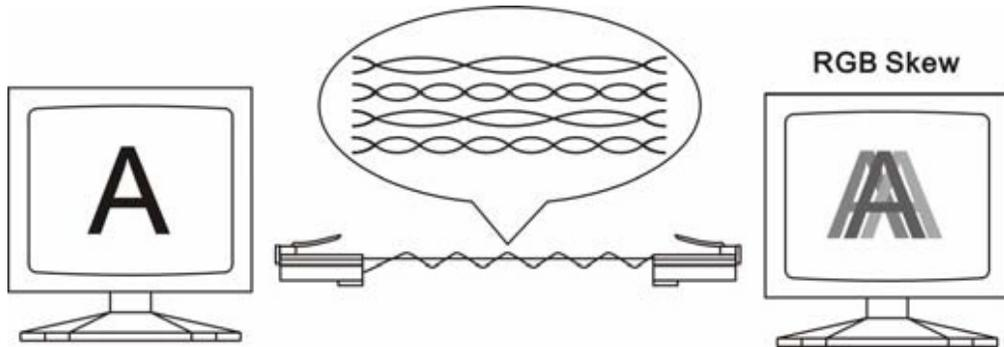
2. Recommend to use following cabling design to reduce skew status, and to add special made "skew immunized adaptor" (2 pieces included at the package).
