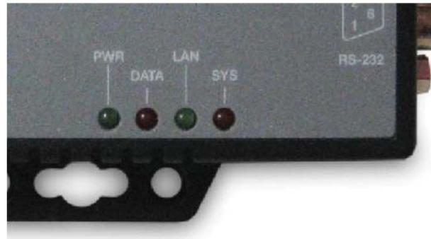
**SYS “Red LED”** : Power indicator (When power on, LED will flash each time in one second.)
