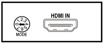
HDMI IN: Connects to an HDMI source with an HDMI Male-Male cable here
