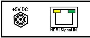
**HDMI Signal IN**: Plug in a CAT-5/5e/6 cable that needs to be linked to the RJ-45 connector of the Sender unit AT-HD-V40SS. **+5V DC**: Connect to 5V DC power supply.
