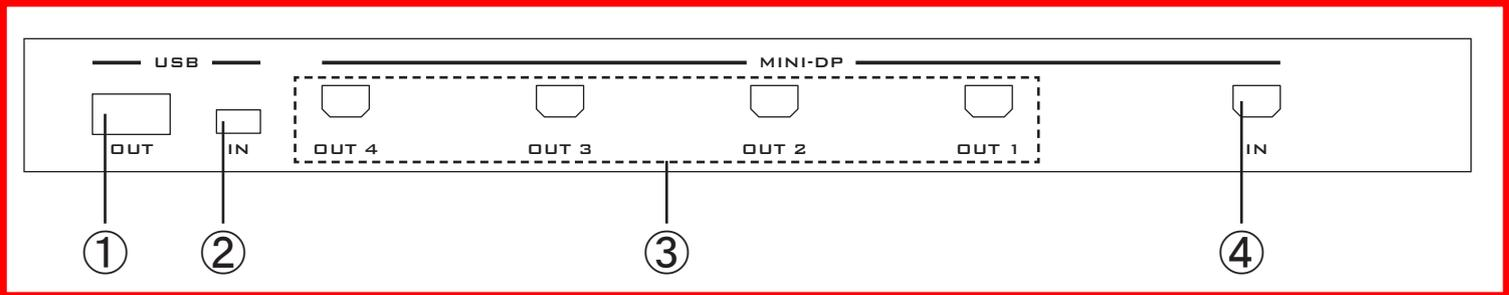
1. USB OUT: Connect a USB A type cable to the display monitor or PC/notebook for audio & USB signal bypass. There is only 1 x USB by-pass, all the other displays USB connections should be connected directly to the computer.
