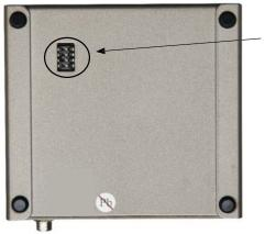
Exposed DIP Switch Bank Underneath the Sender and Receiver units
