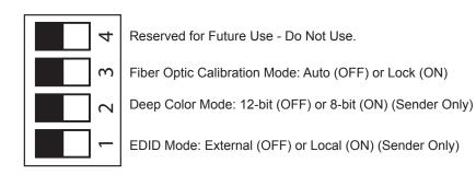
To make changes to the settings, move the appropriate DIP switch to its ON or OFF position. Use an object with a small point such as a mechanical pencil with the lead retracted or a very small screwdriver.
