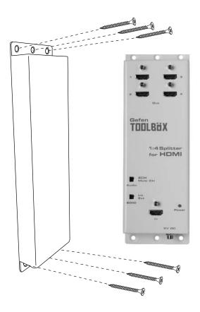
The GefenToolBox 1:4 Splitter for HDMI 1.3 should be mounted vertically in a wall or cabinet with wood/drywall screws as shown in the diagram above. There should be an inch or two of clearance between the edges of the unit and any walls or vertical surfaces to allow for enough clearance for insertion and retraction of cables at the HDMI connectors.
