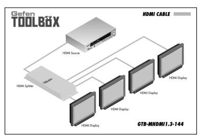
Wiring Diagram for the GefenToolBox 1:4
