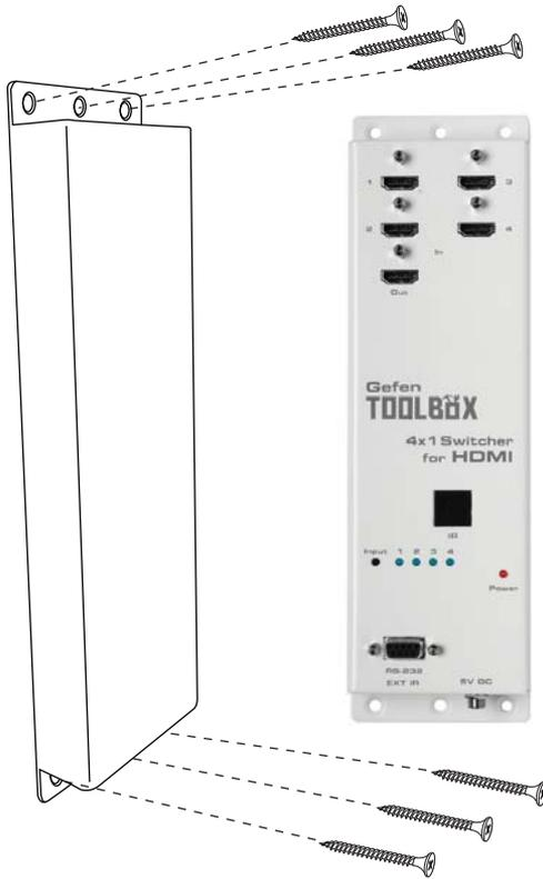
The Gefen Toolbox 4x1 Switcher for HDMI 1.3 should be mounted vertically in a wall or cabinet with wood/drywall screws as shown in the diagram above. There should be an inch or two of clearance between the edges of the unit and any walls or vertical surfaces to allow for enough clearance for insertion and retraction of cables at the HDMI connectors.
