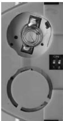
Left: Picture of the opened rear battery compartment of the IR remote showing the exposed DIP Switch bank between the battery chambers.
