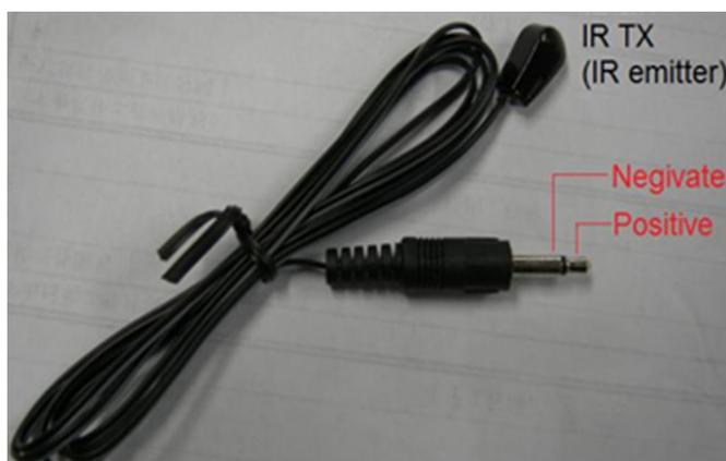
*Note: For better functionality of the IR, we suggest to place the IR receiver Eye at the IR Eye of the controlling source.*
