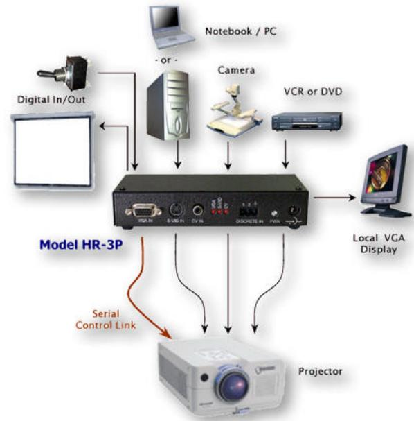
Typical Setup Block Diagram
