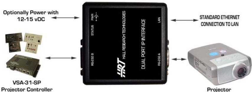
Figure 1 – Typical Setup
