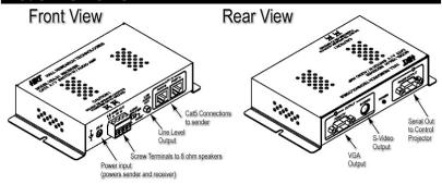
As seen in the above diagrams, the connection between the receiver and the projector could be comprised of VGA, S-Video, and RS232. These cables are not supplied and must be purchased separately.
