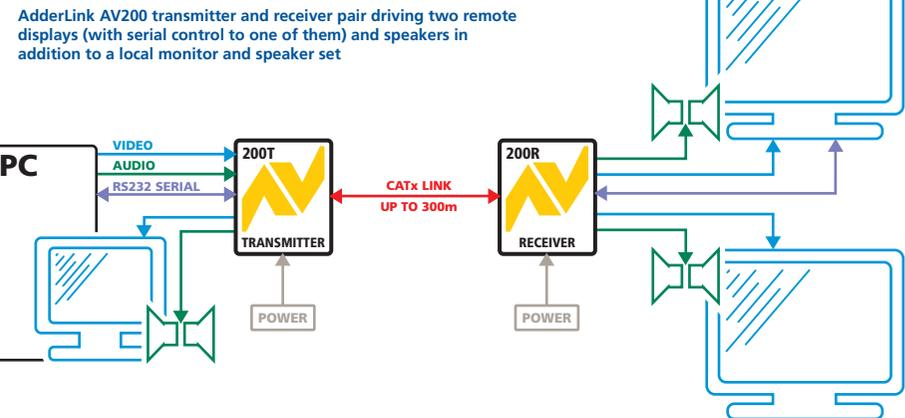
The AV200P transmitter and receiver modules are also available separately and are known as the AV200T and AV200R respectively. Expansion is made possible by connecting further transmitters to the original AV200T transmitter module, however, the serial connection cannot be cascaded in this manner. Where cascades with serial connections (as well as video and audio) are required, use the AV204T/AV208T transmitters.
