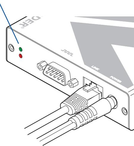
Indicator positions on AV204T and AV208T units
