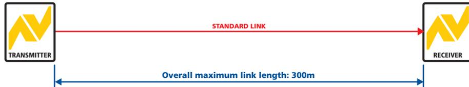
*Note: Long cable lengths may induce colour separation effects. AdderLink AV201R receivers contain the necessary circuitry to minimise such effects.*
