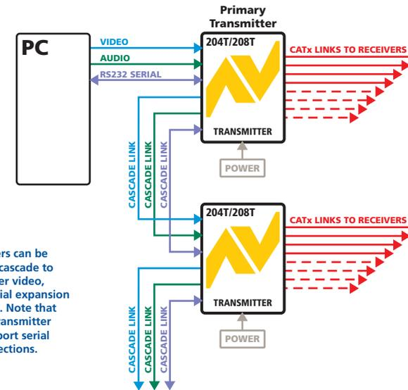
AV transmitters can be connected in cascade to provide further video, audio and serial expansion opportunities. Note that the AV200T transmitter does not support serial cascade connections.
