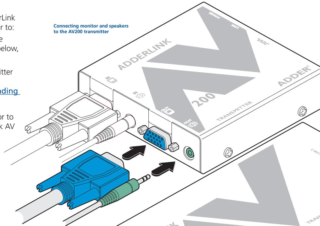
Connecting monitor and speakers to the AV204 or AV208 transmitter
