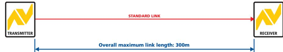
However, if other transmitters are connected in cascade to the initial transmitter, then the overall length of the link cables used must be reduced. For further information, please refer to the section [Making cascade connections](#).
