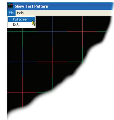
The screen will show a series of fine red, green and blue crosses which should all be in line, vertically and horizontally- skew affects the horizontal placement of the colours.
