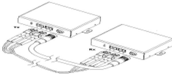
Figure 4 – Connection of 2 duplex LC fiber cables and a DDC cable
