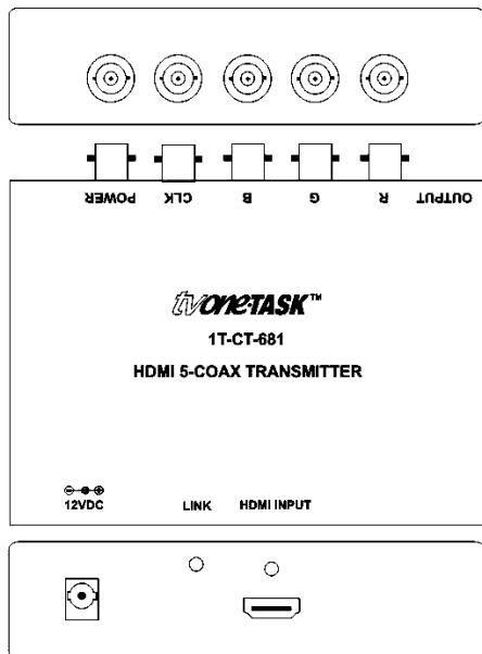
1. Connect the HDMI source device's output to the HDMI IN connector of the 1T-CT-681 Transmitter, using an appropriate HDMI cable, (3 Meter (~9') in length for 12 bit signals, 6 meters (~18' for 8 bit signals).
