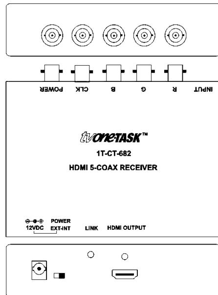
1. At the remote location, connect the RG-6 cables to the appropriate inputs. Do not interchange the cables. The Video cables must be connected to the same video inputs and outputs on both the Receiver and Transmitter and the Clock (CLK) cable must be connected to the Clock connector on both units. If the cable run is less than 180 feet, connect a fifth cable to the connector labeled "Power" but if the cable run is greater than 180 feet, DO NOT connect the fifth cable.
