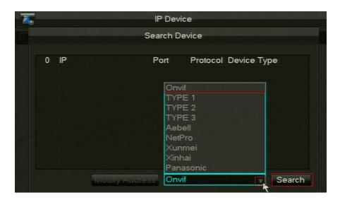
Note: All IC Realtime cameras are Onvif compatible but if using 3<sup>rd</sup> party cameras with the STREAMBOX you will need to select a compatible protocol for each device.
