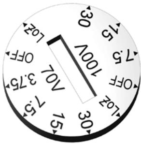
Models with 6-inch and 8-inch drivers are fitted with 60W transformers. In distributed line applications, the transformer can be tapped at 60 W, 30 W and 15 W, with an additional 7.5 W tap for 70 V line systems.
