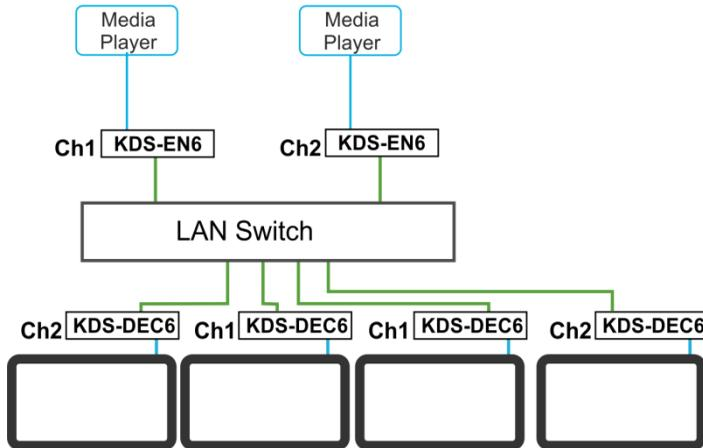
Figure 8: Connecting the KDS-EN6, KDS-DEC6 Video Encoder
