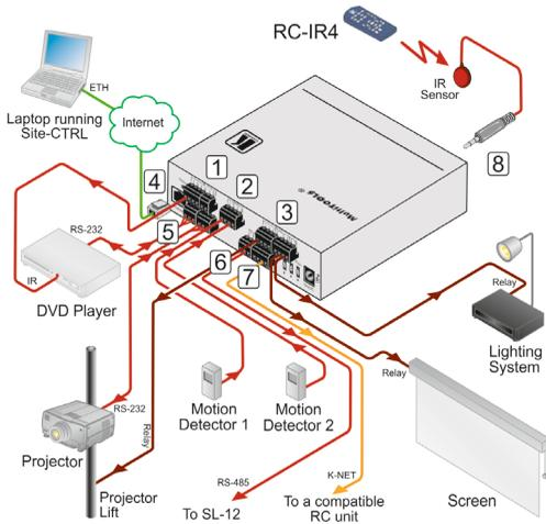
Always switch off the power on each device before connecting it to your **SL-10**.
